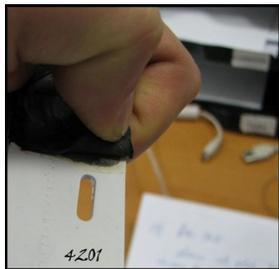
Setting blocks are materials used for the fixation of IG units in the glazing rebate and for the load transfer of the individual glass panes. They should be included in tests because (environmentally friendly) blends of reclaimed material that is currently being used could be incompatible with the sealant system.
